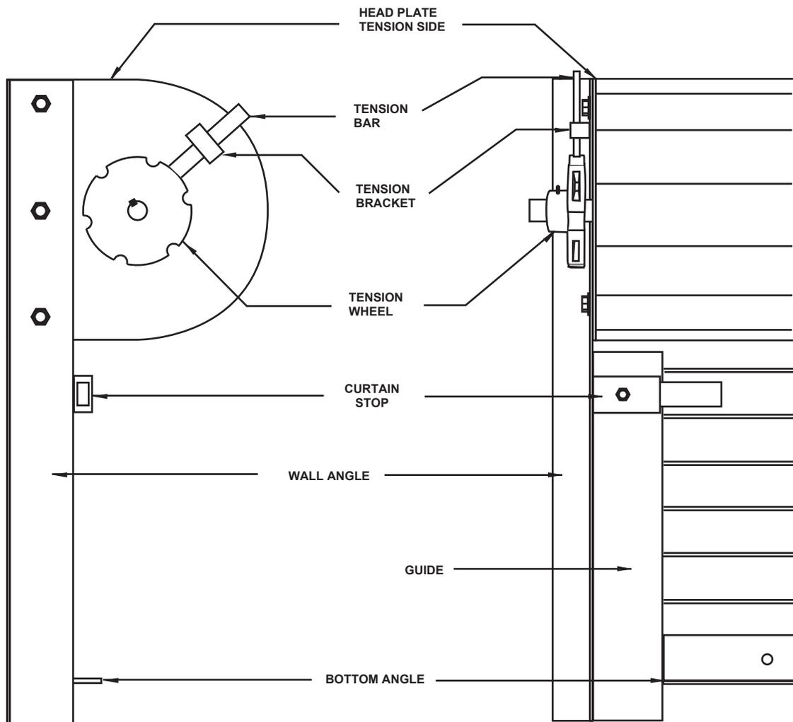
FIGURE 9 TENSION SIDE
